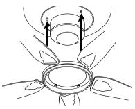
Figure 6c - Attaching Speed Ring™ to Motor
